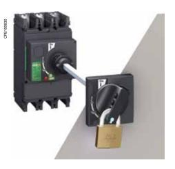
Escutcheons are an optional feature mounted on the switchboard door. They increase the degree of protection to IP40, IK07. Protection collars maintain the degree of protection, whatever the position of the device (connected, disconnected).
